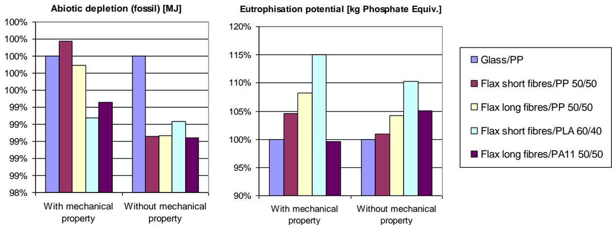
**Figure 3: Abiotic depletion (a) and eutrophication potential (b) for the life cycle of the composites with and without the mechanical property**
