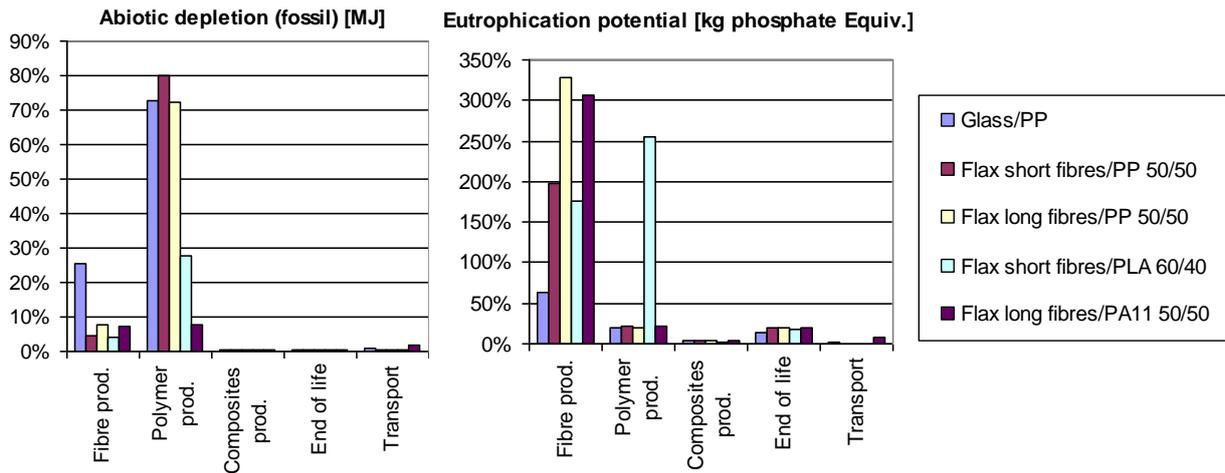
**Figure 2: Abiotic depletion (a) and eutrophication potential (b) for the production phase (fibres, polymers and composites production), the transport and the end-of-life**
