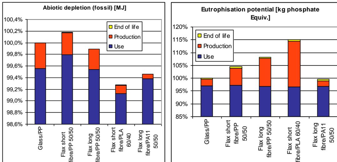
**Figure 1: Abiotic depletion (a) and eutrophication potential (b) for all the life cycle**
